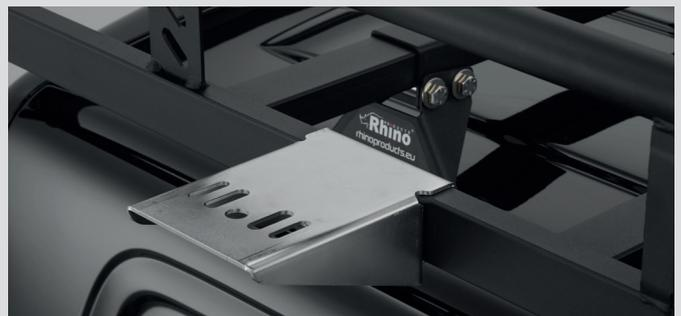
Our side mounting kit is a popular optional extra for the PipeTube Pro. Consisting of two side mounting brackets and all required fixings, this kit allows a 3.0m PipeTube to be mounted to the side of a Rhino ModularRack, enabling full width usage of the rack. One key benefit this provides is the option to transport 8' x 4' boards on the roof of the van, along with the use of a PipeTube.
