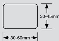
\*The PipeTube Pro can also be used on any other roof bar or roof rack system that fits within these dimensions.
