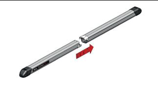
The two 1.5m halves of a 3m PipeTube Pro can then be joined together via a quick and easy assembly process.
