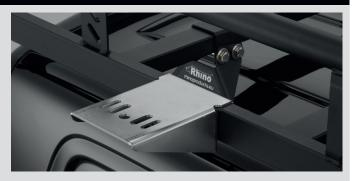
Our side mounting kit is a popular optional extra for the PipeTube Pro. Consisting of two side mounting brackets and all required fixings, this kit allows a 3.0m PipeTube to be mounted to the side of a Rhino ModularRack, enabling full width usage of the rack. One key benefit this provides is the option to transport 8' x 4' boards on the roof of the van, along with the use of a PipeTube.
